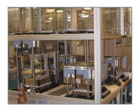
152 x High Pressure Reactors, SS316, Gas Liquid Reactions, 100 bar, 170 C.
