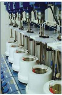
Low Pressure Glass Reactors. For Testing Lubricants, 250 C.
