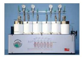
Our Chameleon Range. 4x High Pressure Reactors, Gas/Liquid Reactions, Magnetic Stirring, 30 bar, 120C.
