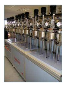
12 x High Pressure Glass Reactors, C276, Hydrogenation and with hydrogen dosing, 200 bar, 250 C.
